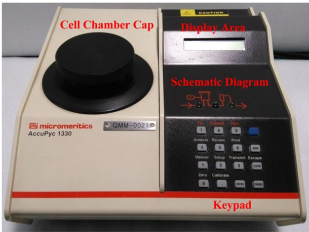
Fig. 8. Automated pycnometer AccuPyc 1330.
